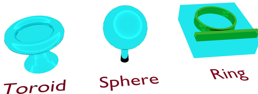
Schematic of typical shapes of microresonators going from the toroid (left) to the integrated ring resonator (right) but also the sphere (center).
